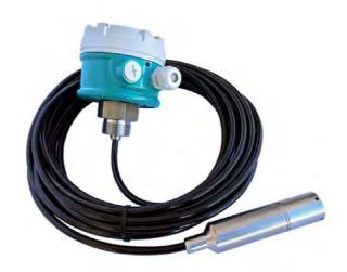
Suitable for continuous liquids level measurement. Typical application are waste water and deep wells. The KP level transmitter configuration options make it suitable for most industrial sectors (oil, chemical, power, metallurgy, pharmaceutical and food) and in different operating conditions. These characteristics make it the ideal instrument in process automation for the hydrostatic head levels measurement.
